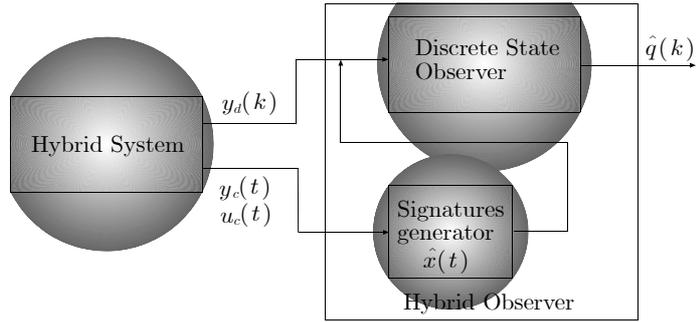
Figure 3.1: Observer structure: location observer and continuous observer
