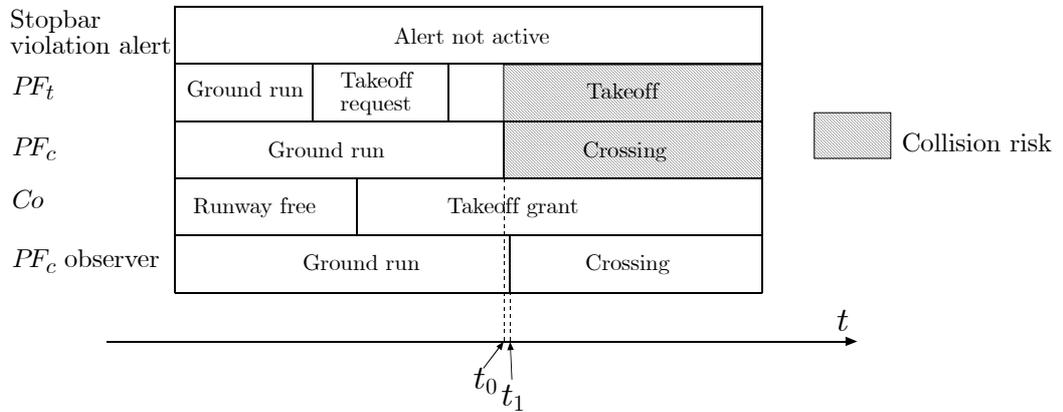
Figure 3.6: Simulation 2 – Stopbar violation system out of service
