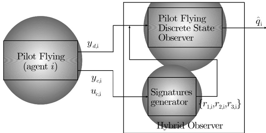
Figure 3.3: Hybrid observer block diagram
