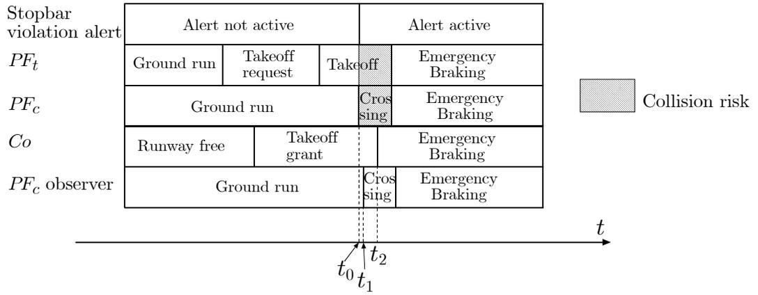
Figure 3.5: Simulation 1 – Stopbar violation system in service
