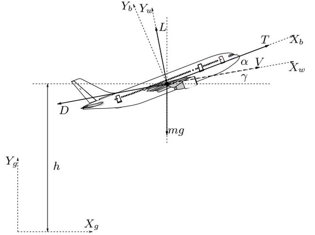
Fig. 1. Coordinate frames and forces for the aircraft model.
